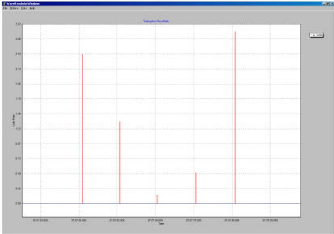
Here are the 50 microsecond and 2 microsecond pulses which show the unit's upper limit:
