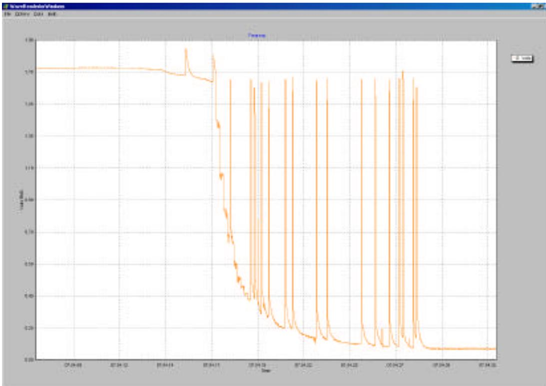
If you watch the computer monitor during logging you should find that at about 4-5 kHz the WaveRider is recording about 1/2 the voltage it did at 45 Hz. The above plot shows how the sensitivity of the WaveRider decreases with frequency. The digitizer in the WaveRider reading causes the numerous “spikes” due to the
