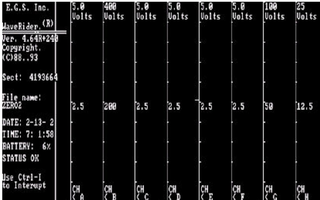
Mr. Pulsar’s output is a square wave of 5.0 volts “peak-to-peak”. When Mr. Pulsar’s square wave output is read by a “true rms” voltmeter, it will read approximately 2.5 volts. When read by the WaveRider, it will read approximately 2.5 volts “peak” or 1.76 volts “rms”. Why is this?
