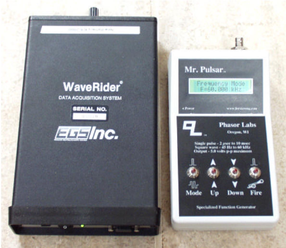
The following application note will show you how to use the Mr. Pulsar unit to field calibrate your WaveRider stray voltage monitor.
