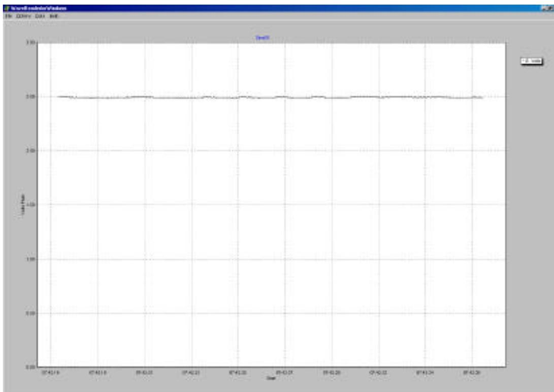
With a 1.76 volt rms 60 Hertz sine wave the “rms” value on the WaveRider should be approximately 1.76 volts as shown below:
