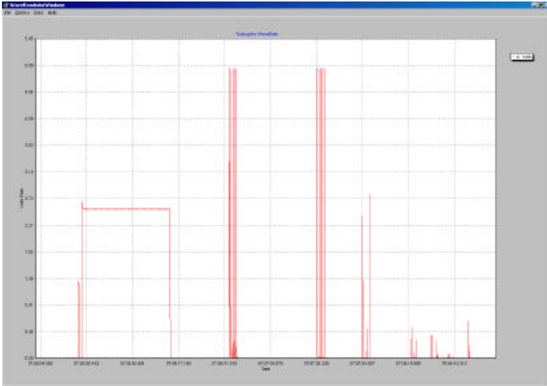
The reason the steady state 60 Hertz voltage level is lower than the pulse magnitudes is that the input DC blocking capacitor averages a steady state voltage about the zero axis, but not the short duration pulses.
