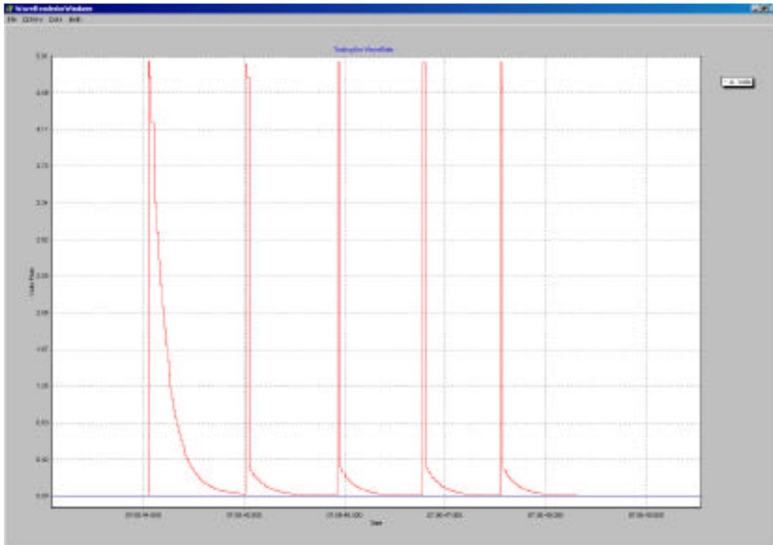
Note the slow decay of the voltage on the first pulse. This is due to the input capacitor. If I delayed sending the pulses, each pulse would have had a similar decay period. This is not important, but I just mentioned it in case you wondered.
