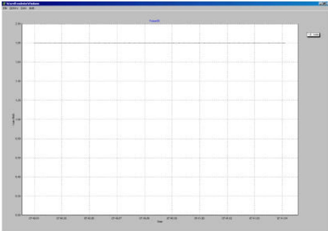
With a 1.76 volt rms 60 Hertz sine wave the “peak” value on the WaveRider should be approximately 2.5 volts as shown below:
