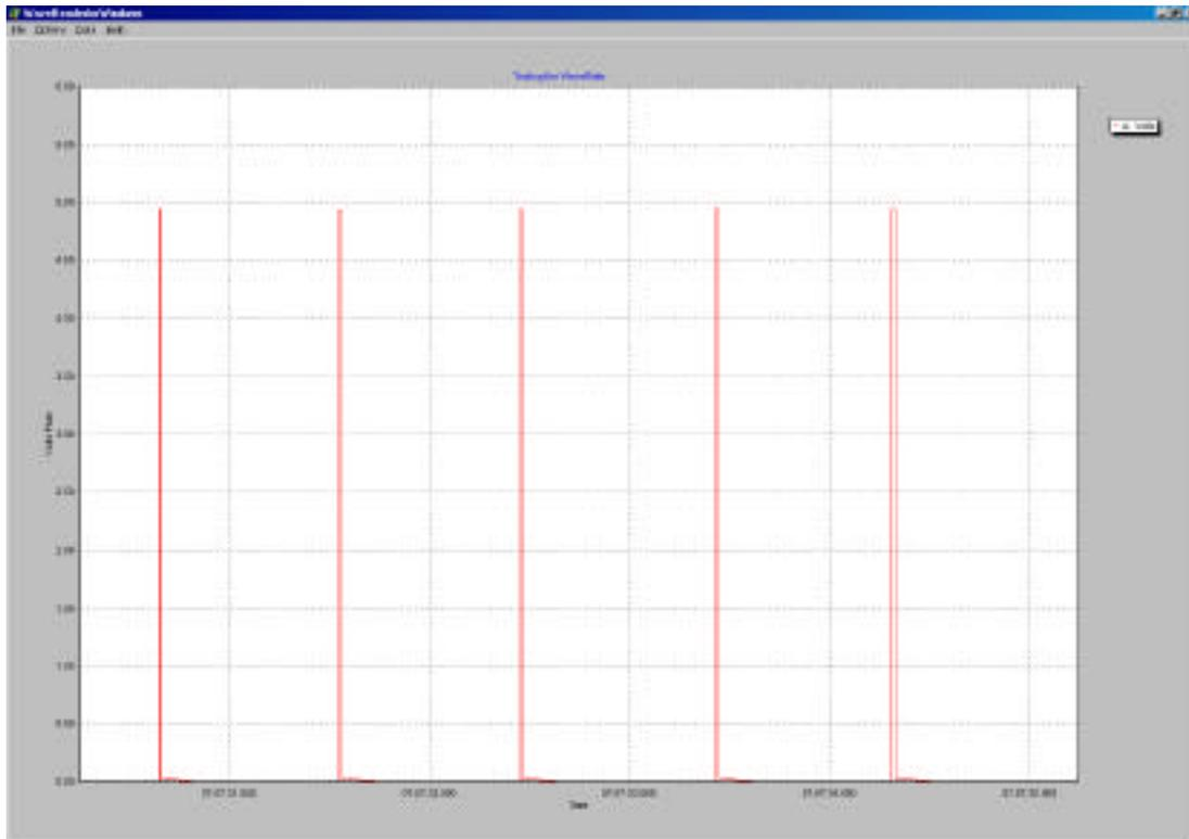
At 1 millisecond, pulses are accurately recorded.
