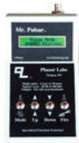
Mr. Pulsar at cow contact R_s = 102 ohms
