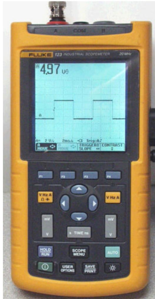
After turning on the unit, push the **Channel A V-Hz-A-ohms-Cap** button.
