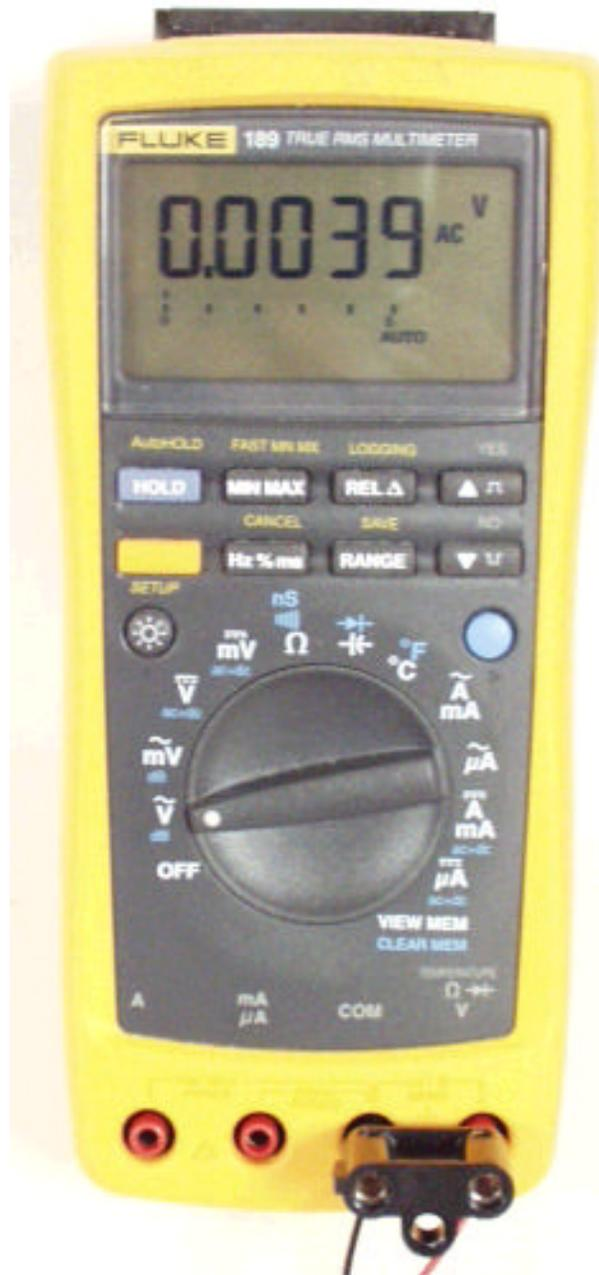
Don't forget to test your meter to make sure when it is in the AC voltage setting it only reads AC volts and not DC. You do have on-farm sources of DC voltage up to 0.6-0.7 volts even when all the power is shut off. We are looking for on and off farm sources of AC voltage. Some meters mix the AC and DC voltages and report them as only AC, this is not correct and is also very confusing when making measurements.
