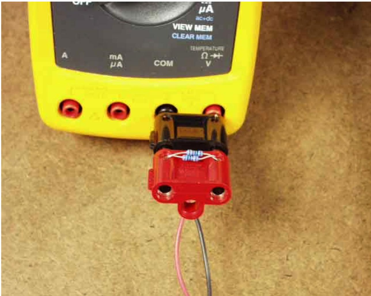
As long as you are to this point, plug ONLY the 500 ohm resistor into the meter, put the meter on the ohms ( $\Omega$ ) scale and measure to make sure your resistor is between 475 and 525 ohms.
