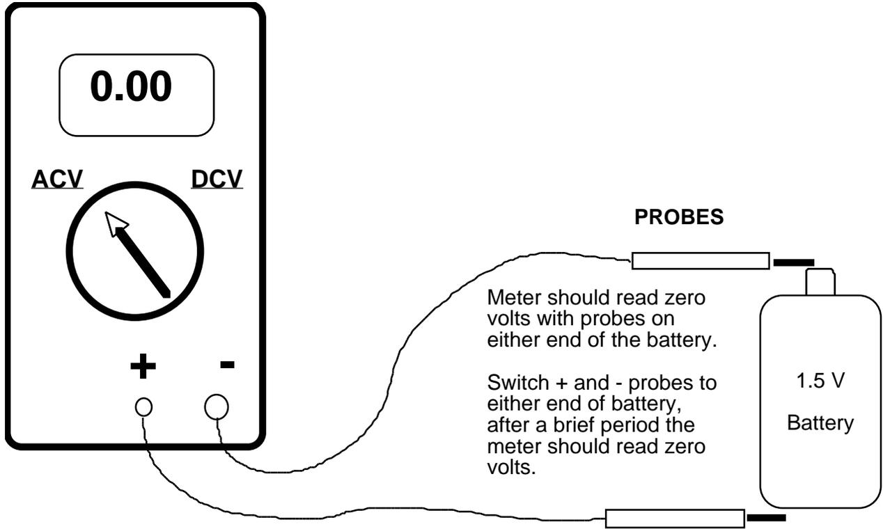
Meter should read zero volts with probes on either end of the battery.
