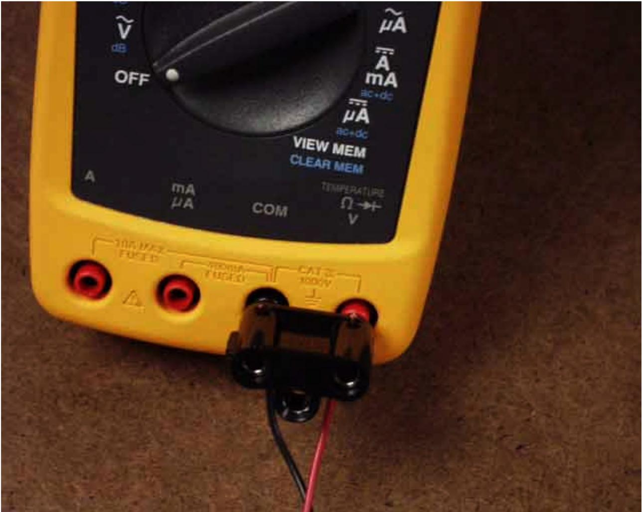
Next take a second banana plug and put a 500 ohm resistor between the terminals. Use two 1/2 watt 1,000 ohm resistors in parallel as shown below. Resistors are available from Radio Shack. Use 1/4 watt or 1/2 watt types. This will be your 500 ohm “Cow Resistor”.
